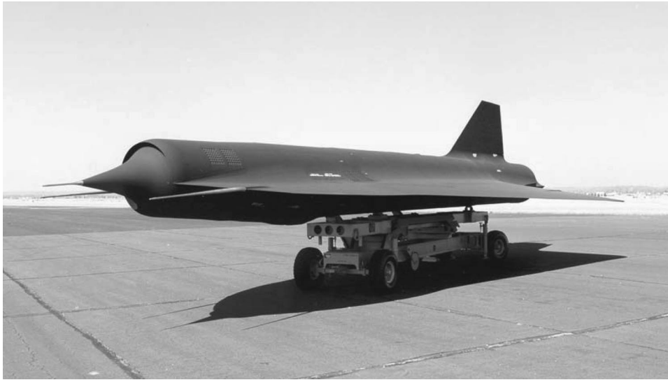
Figure 1.2: Lockheed D-21B unmanned reconnaissance aircraft. ( Courtesy of the National Museum of the USAF. )
